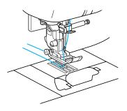
Reattach the bobbin cover. Insert the tab in the lower-left corner of the bobbin cover, and then lightly press down on
